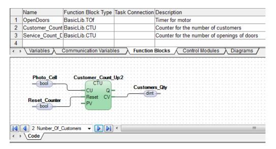
Figure 28. .Variable connections to Customer\_Count\_Up Function Block Type
