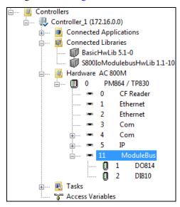
Figure 35. Hardware setup (Project Explorer).
