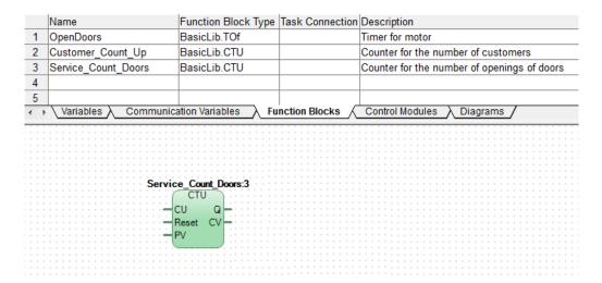
Figure 26. Declare CTU Function Block Type in Service\_On\_Doors page
