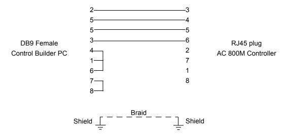
Figure 74. Cable TK212A Pinout configuration.
