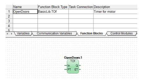
Figure 24. Declare TOf Function Block Type in Motors\_Doors page
