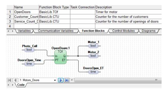
Figure 27. Variable connections to OpenDoors Function Block
