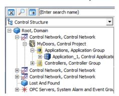
Figure 56. Control Structure view. Note that Control Network and MyDoors project have been added to the Control Structure by Control Builder.
