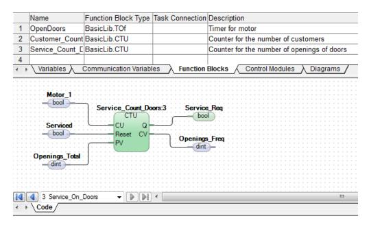
Figure 29. Variable connections to Service\_Count\_Doors Function Block Type
