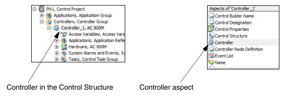
Figure 69. (Left) Selected controller in the Control Structure. (Right) The Controller aspect for the selected controller (Controller\_1).
