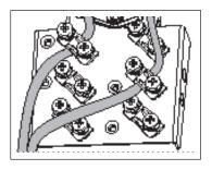
7. Connect the conductors to the appropriate detachable terminals of the control unit. See chapter *Control unit (page 107)* for the default I/O connections of the drive module. Use shrink tubing or insulating tape to contain any stray strands. Tighten the screws to secure the connection.
