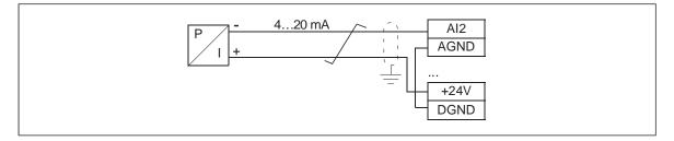
An example of a three-wire sensor/transmitter supplied by the drive auxiliary voltage output is shown below. The sensor is supplied through its current output and the drive feeds the supply voltage (+24 V DC). Thus the output signal must be 4...20 mA, not 0...20 mA.
