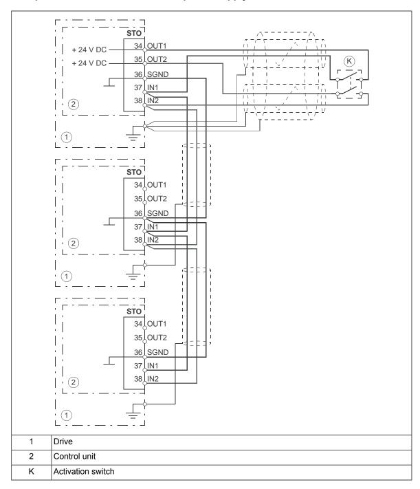
Multiple ACQ580-04 drives, internal power supply
