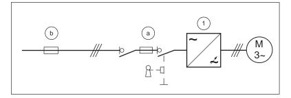
Size the fuses or the circuit breaker according to local regulations for the input cable protection. Select the fuses for the drive according to the instructions given in the technical data. The fuses for the drive protection will restrict drive damage and prevent damage to adjoining equipment in case of a short-circuit inside the drive.
