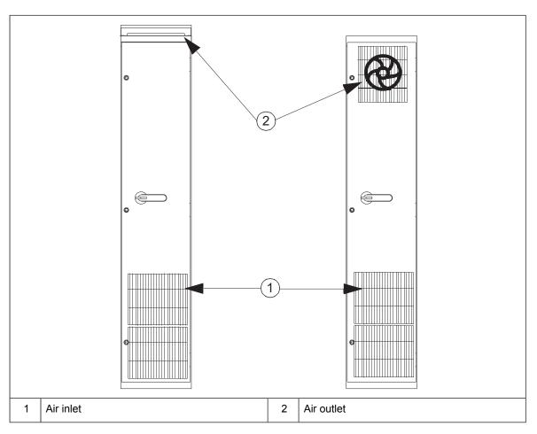
Note: Use an extra exhaust fan if the air outlet is on the cabinet door.
