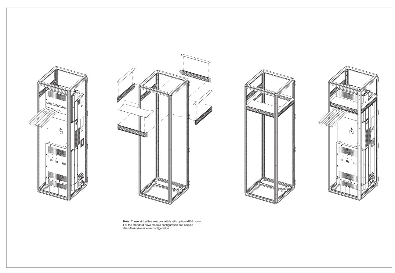
**Note:** These air baffles are compatible with option +B051 only. For the standard drive module configuration, see section *Standard drive module configuration (page 29)*.
