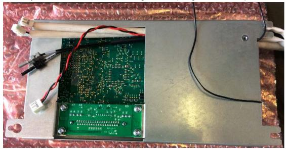
4. Connect the cables to their connectors on the ZBIB board.
