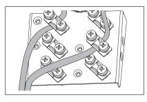
11. Connect the conductors to the appropriate detachable terminals of the control unit. See the default I/O diagram in chapter *Control unit (page 107)*. Use shrink tubing or insulating tape to contain any stray strands. Tighten the screws to secure the connection.
