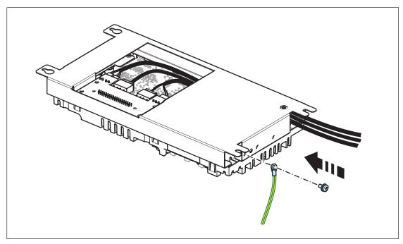
6. The kit includes a plate for the customer cable screens. Attach the small bracket (a) first, then the full clamp plate (b).
