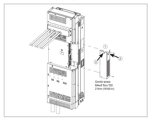
3. Connect the control cables to the drive module . Make sure that that cables are not against sharp edges or bare live parts
