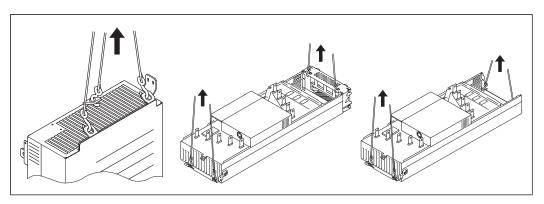
Make sure that the module does not topple over when you move it on the floor: Open the support legs by pressing each leg a little down (1, 2) and turning it aside. Whenever possible attach the module also with chains. Do not tilt the module. It is heavy and its center of gravity is high. The module overturns from a sideways tilt of 5 degrees. Do not leave the module unattended on a sloping floor.
