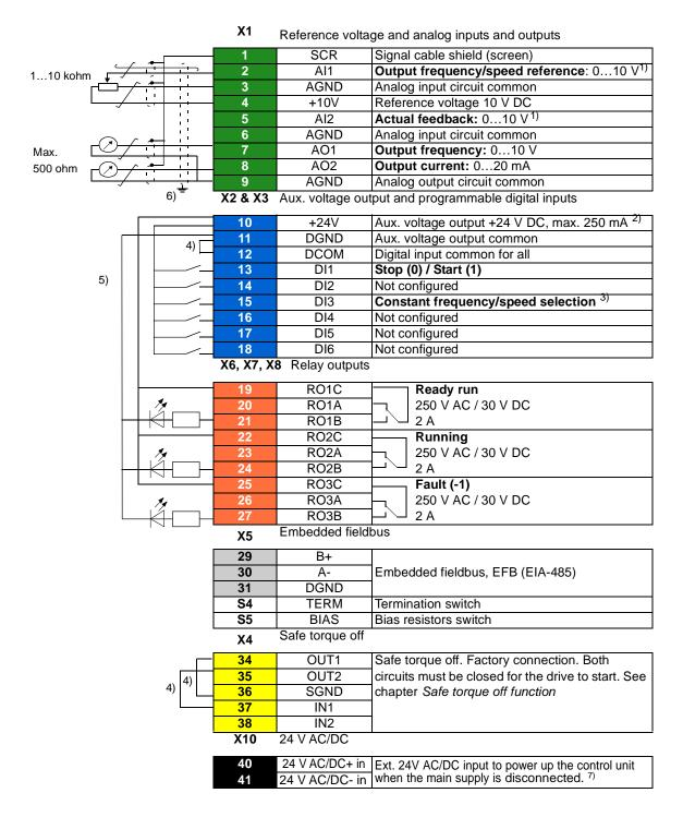
Total load capacity of the Auxiliary voltage output +24V (X2:10) is 6.0 W (250 mA / 24 V DC). Digital inputs DI1...DI5 also support 10 to 24 V AC Terminal sizes: 0.14...2.5 mm<sup>2</sup> (all terminals) Tightening torques: 0.5...0.6 N·m (0.4 lbf·ft) **Notes:**
