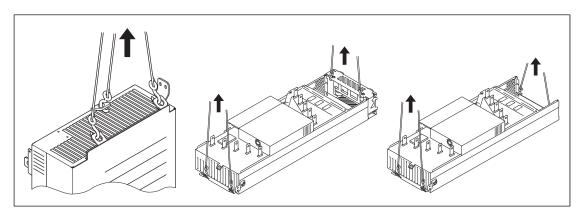
Make sure that the module does not topple over when you move it on the floor: Open the support legs by pressing each leg a little down (1, 2) and turning it aside. Whenever possible attach the module also with chains. Do not tilt the drive module. It is heavy and its center of gravity is high. The module overturns from a sideways tilt of 5 degrees. Do not leave the module unattended on a sloping floor.
