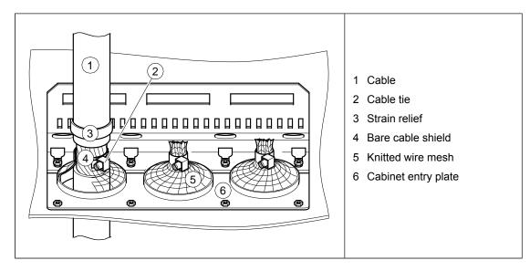
ABB recommends 360° high-frequency grounding of the control cable shields at their entries. The shields can be grounded by means of conductive shielding cushions pressed against the cable shield from both directions as shown below.
