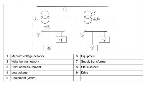
2. An EMC plan for preventing disturbances is drawn up for the installation. A template is available in *Technical guide No. 3 EMC compliant installation and configuration for a power drive system* (3AFE61348280 (English)).
