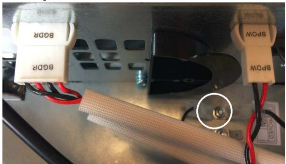
4. Connect the ground connection at the drive module end.
