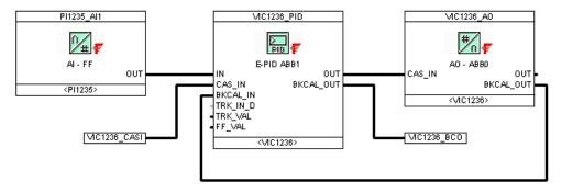
Figure 2. Fieldbus Builder FF - Cascaded PID Loop, Slave PID
