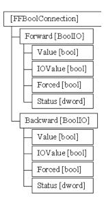
Figure 23. FFBoolConnection Data Type Structure
