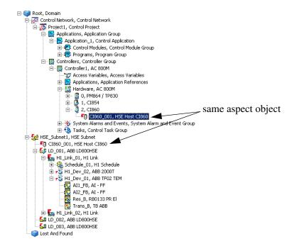
Figure 11. Control Structure with Control Network and HSE subnet
