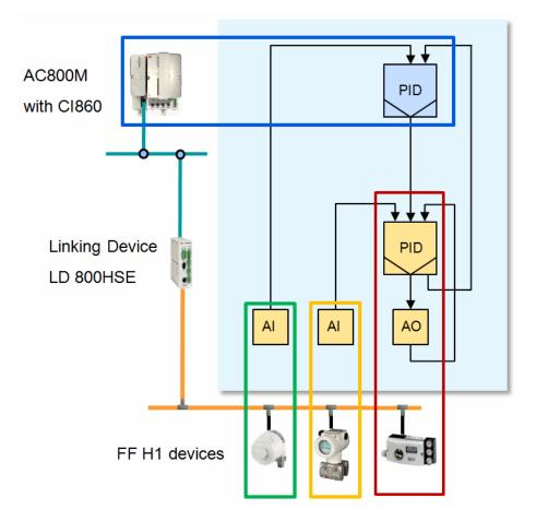
*Figure 1. Sample Cascaded Control Loop Running Distributed on FF and on AC 800M Controller*
