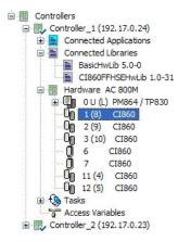
Figure 9. Redundant CI860 in Hardware Tree
