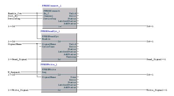
Figure 11. Control Builder Function Block Diagram for C/S access
