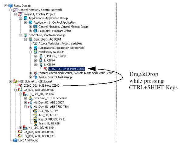
Figure 12. Create Reference of the HSE Host CI860 Object
