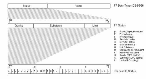
Figure 2. Status Handling for Inputs
