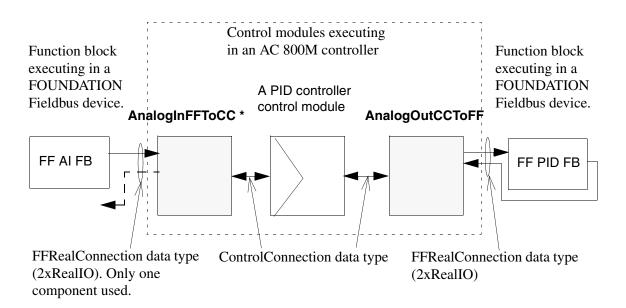
\* can be omitted by using the CI860 channel directly (RealIO) since no backward signal is used
