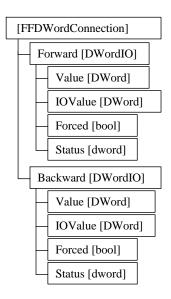
Figure 24. FFDWordConnection Data Type Structure
