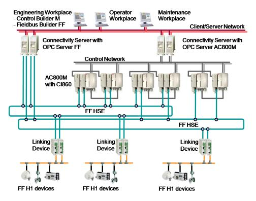
Figure 1. System 800xA topology with FF HSE
