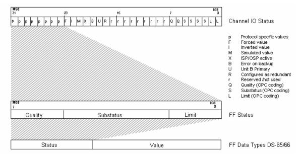
Figure 3. Status Handling for Outputs
