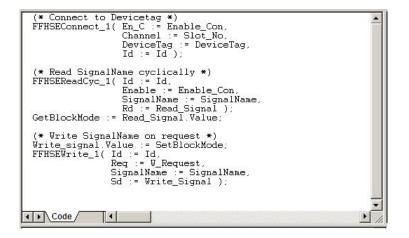
Figure 13. Control Builder Structured Text sequence for C/S access
