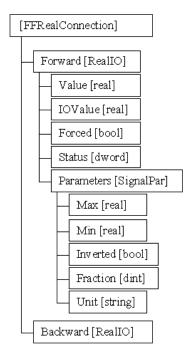
Figure 19. FFRealConnection Data Type Structure
