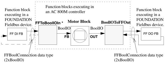
\* can be omitted by using the CI860 channel directly (BoolIO) since no backward signal is used.
