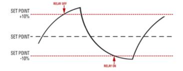
**Note:** The continuous zero and span points and the Switch Configuration Mode and set point(s) must be specified. Refer to switch configuration diagrams on page 3.
