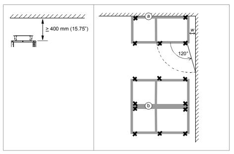
**Note 1:** Any height adjustment must be done before attaching the cabinet sections to the floor or to each other. Height adjustment can be done by using metal shims between the cabinet bottom and floor.
