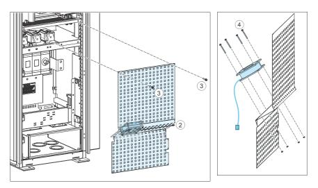
Replacing the door fan (frames R10 and R11)
