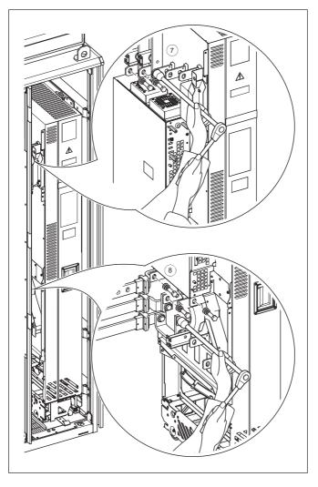
8. Disconnect the drive module output busbars. M12, 70 N·m (52 lbf·ft).
