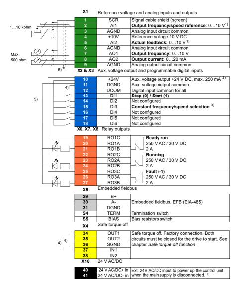
Total load capacity of the Auxiliary voltage output +24V (X2:10) is 6.0 W (250 mA / 24 V DC).
