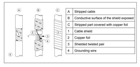
**Note for top entry of cables:** When each cable has its own rubber grommet, sufficient IP and EMC protection can be achieved. However, if there is more than one cable per grommet, plan the installation beforehand as follows:
