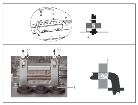
**Note 1:** Keep the shields continuous as close to the connection terminals as possible. Secure the cables mechanically at the entry strain relief.
