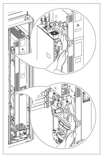
8. Disconnect the drive module output busbars. M12, 70 N·m (52 lbf·ft).
