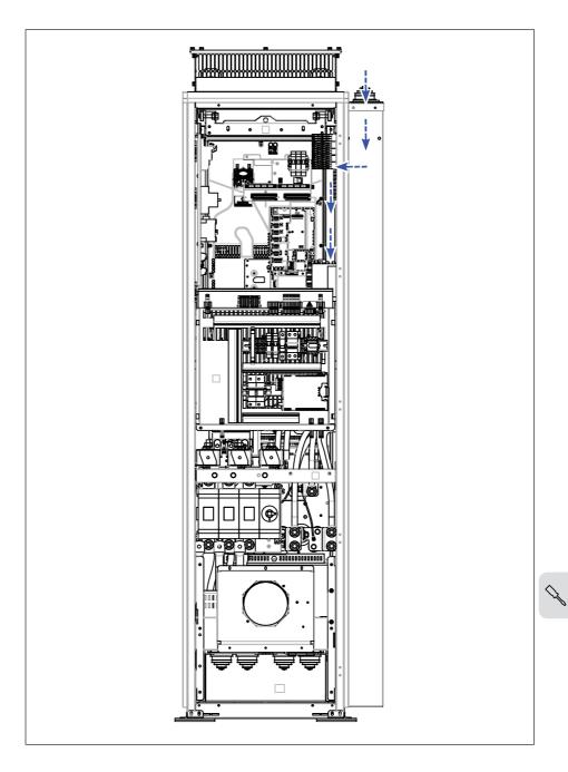
The route of the control cables for frames R10 and R11 is shown below.
