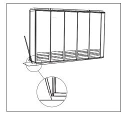
Move the cabinet into its final position with an iron bar. Place a wooden piece at the bottom edge of the cabinet in order not to damage the cabinet frame with the iron bar.
