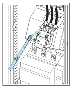
12 Disconnect the input power cable conductors and motor cable conductors from the drive module terminals.
