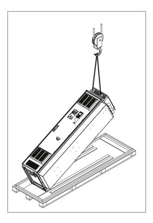
Lift the cabinet to its position. Maximum allowed angle of the lifting slings is  $20^{\circ}$  ( $10^{\circ}$  for frames R10 and R11, IP54).
