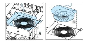
Replacing the drive module main fans (frame R9)
