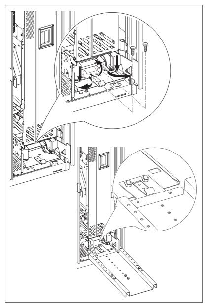
10. Attach the extraction ramp to the cabinet base with two screws.
