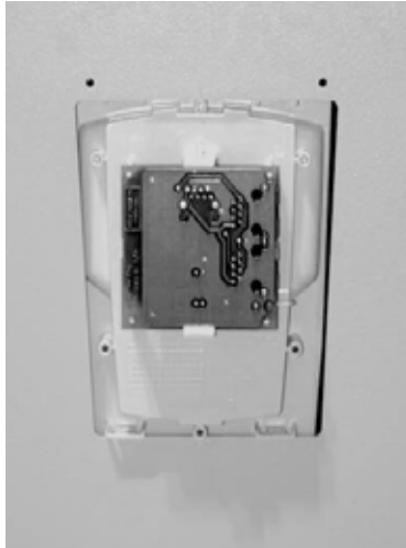
7. Insert the Panel Platform in the hole.
