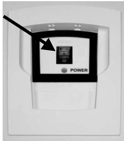
11. Plug in the panel connector supplied with the kit into the socket as shown above.
