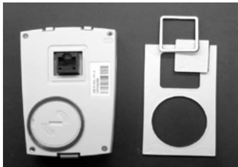
4. Separate square gasket from middle section.
