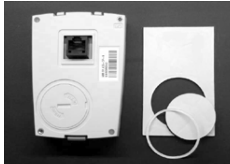
2. Turn your Operator Panel face down and separate ring gasket from middle section.
