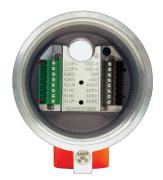
Figure 11 - CLASSIC 800 **Mounting Base Plate / Wiring Terminal**
