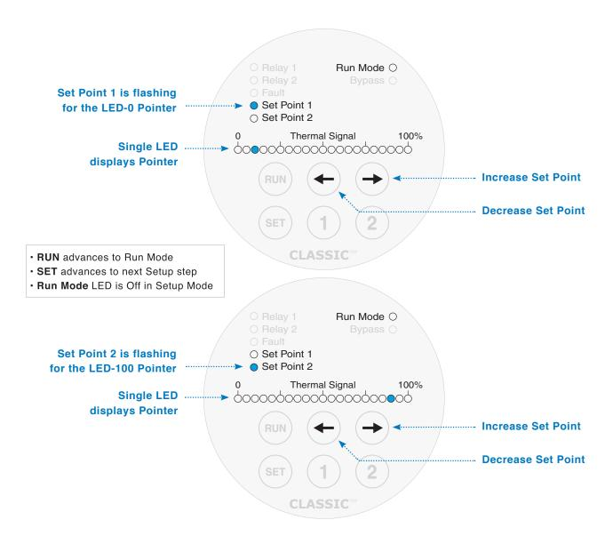
Figure 23 - Setting the 0% & 100% Thermal Signal
