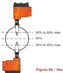
Figure 6b - Horizontal Pipe, **Top / Bottom Mounting**
