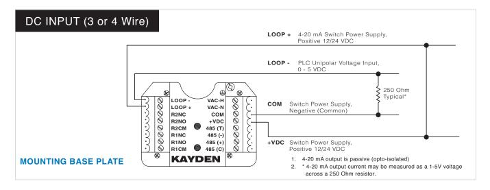
Figure 3 - 4-20 mA Wiring
