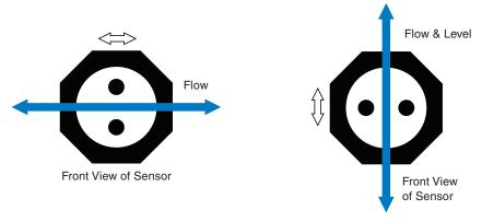
Figure 9 - Sensor Orientation for Horizontal Flow & Level
