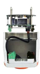
Figure 10 - Disconnecting Sensor Connector from the Electronics Module
