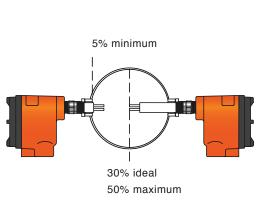
Figure 6a - Horizontal Pipe, **Side Mounting**
