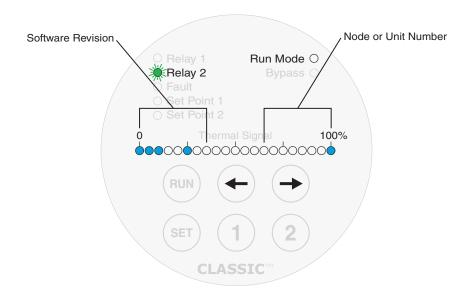
Figure 20 - Software Revision & Node (Unit) Number
