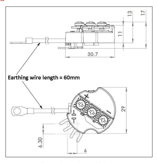
**Figure 3 - Lightning Protector Dimensions**
