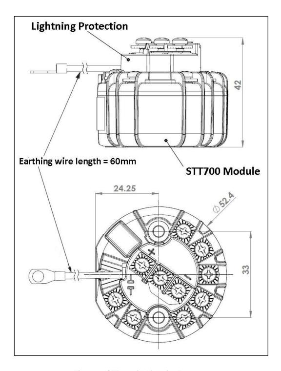
Figure 4 – STT700 with Lightning Protector
