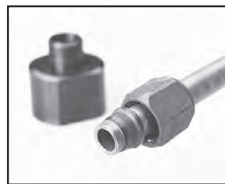
Step 8 – Loosen nut and check for proper pre-set. Use the following inspection criteria.
