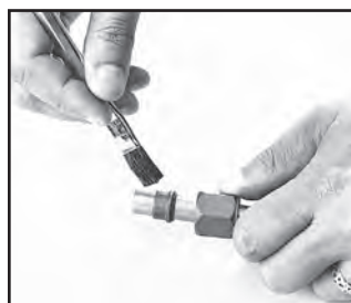
Step 3 – Lubricate ferrule with system fluid or a compatible lubricant. This ensures that the tooling won't stick to the ferrule.
