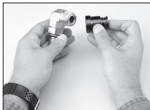
Fig. R25 – O-Ring installation using the CORG assembly tool
