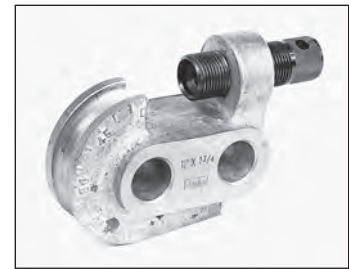
Fig. Q28 — Close Bend Radius Block
