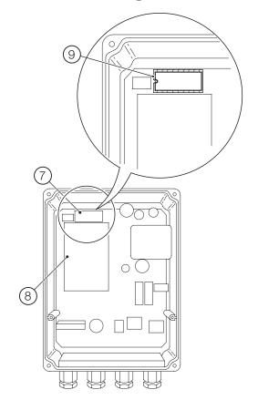
Figure 2 Replacing the EPROM - wall-mount transmitter
