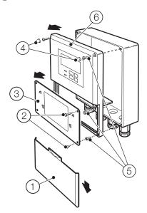
Figure 1 Removing the front cover – wall-mount transmitter
