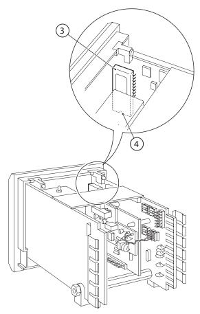
Figure 4 Replacing the EPROM – panel-mount transmitter
