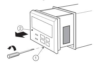
Figure 3 Removing the transmitter from its case
