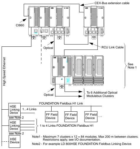
Figure 2.9: Example of AC 800M / S800 I/O and FOUNDATION Fieldbus High Speed Ethernet Interconnection in Redundant CPU Configuration
