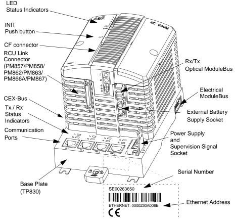
Figure 2.1: Processor Unit - General View
