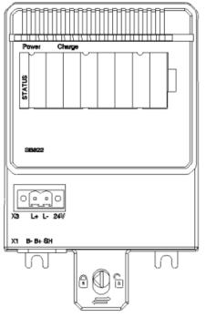
Figure 4.7: SB822 External Rechargeable Battery Unit
