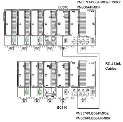
Figure 4.5: Redundant Communication Interface Units and Controllers
