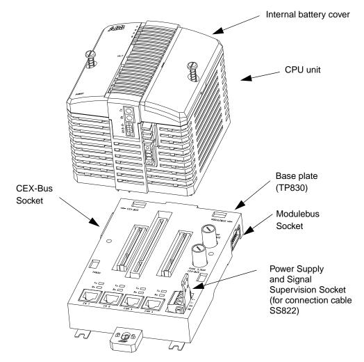
Figure 4.1: Processor Unit Assembly - General View
