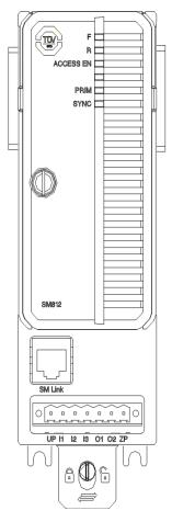
The prime function of SM812 is to provide intelligent supervision of a controller during non-SIL and SIL1-2 operations, and together with a PM857/PM863/PM867 form a 1002 diverse structure for SIL3 applications.
