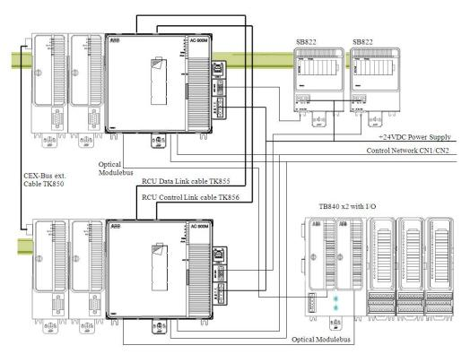
Figure 4.4: Example of Connection of CPU redundancy for PM891
