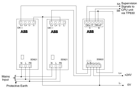
Figure 2.5: Example of a Redundant Power Supply Configuration
