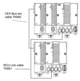
Figure 4.3: Connection of CPU Redundancy
