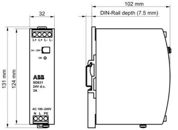
Figure 4.8: SD831 Dimension and Connections for 3 A Power Supply
