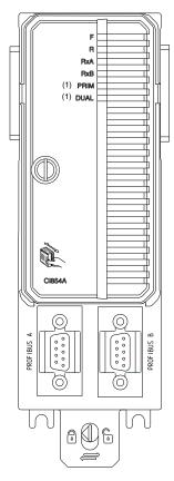
The CI854A/CI854B and TP854 assemblies are used for connecting remote I/O and fieldbus instruments via PROFIBUS DP. The TP854 base plate has two female DB9 connectors for connecting PROFIBUS DP with support of Line Redundancy. The base plate has a preset, two letter Alpha code lock, to prevent the installation of an incorrect type of unit onto the TP854 base plate.
