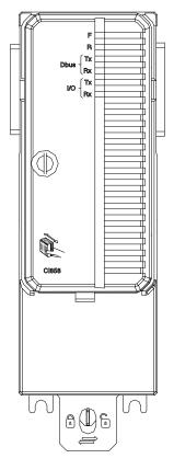
Front View CI858/TP858 The CI858 has three optical connectors. DriveBus connector for connection of ABB Drives, I/O connection, and a Tool connection for downloading firmware to the communication unit with the ABB Drives tools DriveDebug or DriveWindow.
