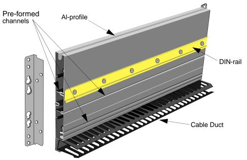
Figure 2.12: Al-profile for DIN-rail support
