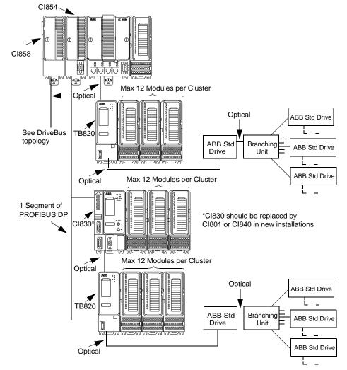
Figure 2.10: Example of Connection of ABB Drives in Single CPU Configuration
