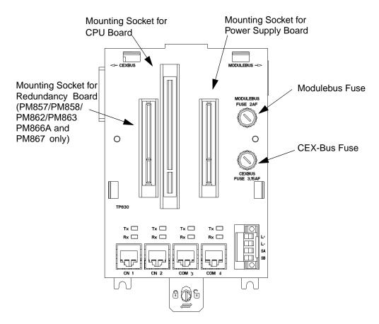
Figure 6.1: TP830 Base plate - Mounting Sockets and Fuses
