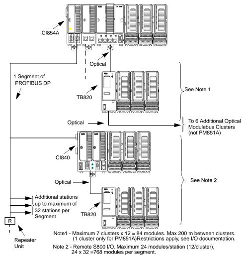
Figure 2.6: Example of AC 800M / S800 I/O Interconnection in Single CPU Configuration
