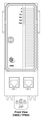
The CI855 and TP853 assemblies are used for connection of an AC 800M to single or redundant MasterBus 300 Networks. This allows DataSet communication and transmission of time between Advant Controller 410/450 and AC 800M.
