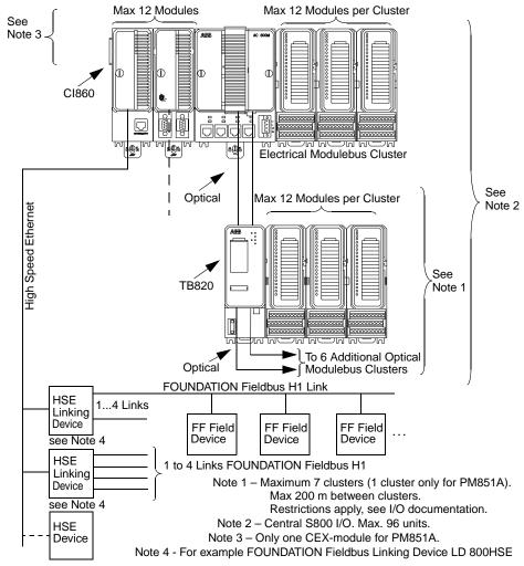
Figure 2.8: Example of AC 800M / S800 I/O and FOUNDATION Fieldbus High Speed Ethernet Interconnection in Single CPU Configuration
