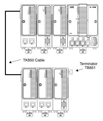
Figure 4.14: TB851 Terminator for CEX-Bus (Female)
