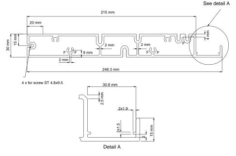
Figure 6.2: AI-Profile for DIN-rail - Dimension Drawing
