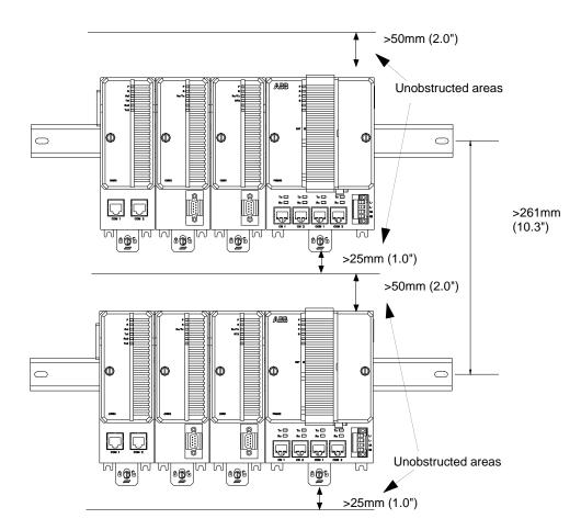
Figure 5.4: Ventilation Requirements - Minimum Mounting Dimensions
