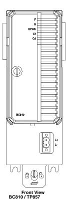
The BC810 CEX-Bus Interconnection Unit offers a way to section the CEX-Bus into two independent segments. This improves availability in systems with redundant communication interfaces. Figure 4.5 on page 56 shows a configuration example. The base plate has a preset, two letter Alpha code lock to prevent the installation of an incorrect type of unit onto the TP857 base plate.
