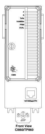
The CI860 / TP860 assemblies are used for connecting FOUNDATION Fieldbus High Speed Ethernet (FF HSE) devices to the AC 800M. It is also possible to communicate with FOUNDATION Fieldbus H1 devices, via the HSE Linking Device (LD 800HSE), see Appendix B, Recommended Components. FF HSE has a communication speed of 10/100 Mbit/s.
