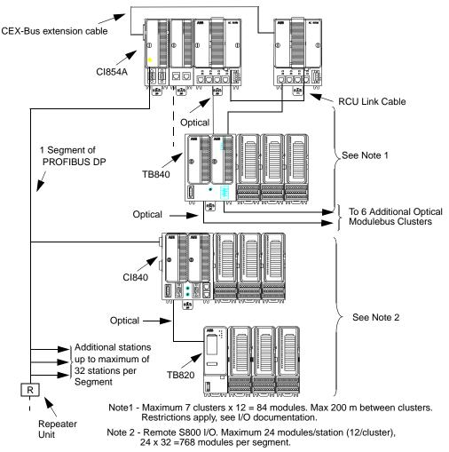
Figure 2.7: Example of AC 800M / S800 I/O Interconnection in Redundant CPU Configuration
