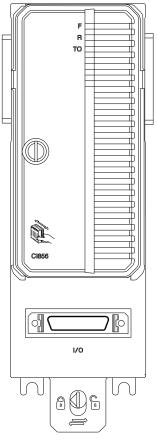
Front View CI856 / TP856 The Cl856 and TP856 assemblies are used for connecting S100 I/O to AC 800M. The TP856 base plate has one female 36 pin center line miniature ribbon connector, for connecting the TK575/TK580 bus extension cable from S100 I/O. A bus extender, DSBC174/DSBC176 or DSBC173A, must also be used. The base plate has a preset, two letter Alpha code lock to prevent the installation of an incorrect type of unit onto the TP856 base plate.
