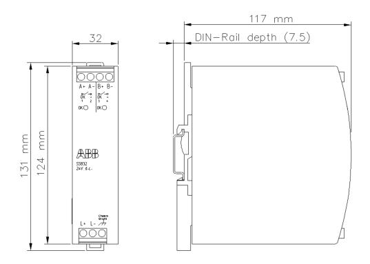
Figure 4.10: SS832 Voting Unit Dimensions and Connections
