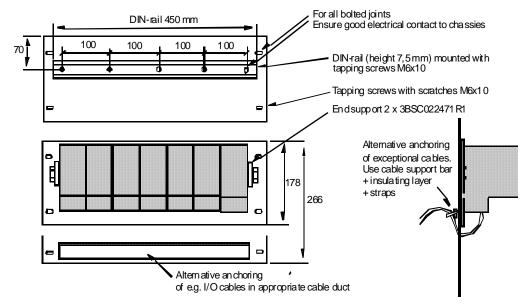
Figure 2.13: Mounted on Metal Sheet
