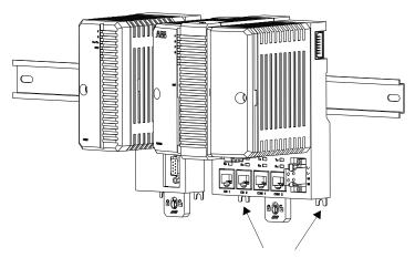
Lugs for extra screws to provide secure mounting in locations subject to vibration
