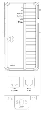
The CI873 is an AC 800M communication interface that connects to external Ethernet devices using the EtherNet/IP protocol.
