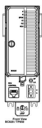
The BC820 CEX-Bus Interconnection Unit offers a way to section the CEX-Bus into two independent segments. This improves availability in systems with redundant communication interfaces. Figure 4.6 on page 58 shows a configuration example. The base plate has a preset, two letter Alpha code lock to prevent the installation of an incorrect type of unit onto the TP850 base plate.
