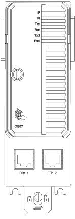
Front View CI857 / TP853 The CI857 and TP853 assemblies are used for connection of an AC 800M controller with INSUM through TCP/IP over Ethernet and an INSUM TCP/IP Gateway which has a LON interface communicating with the underlying INSUM system.
