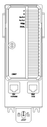
The CI867/TP867 is used for connection between an AC 800M controller and external Ethernet devices using Modbus TCP protocol.
