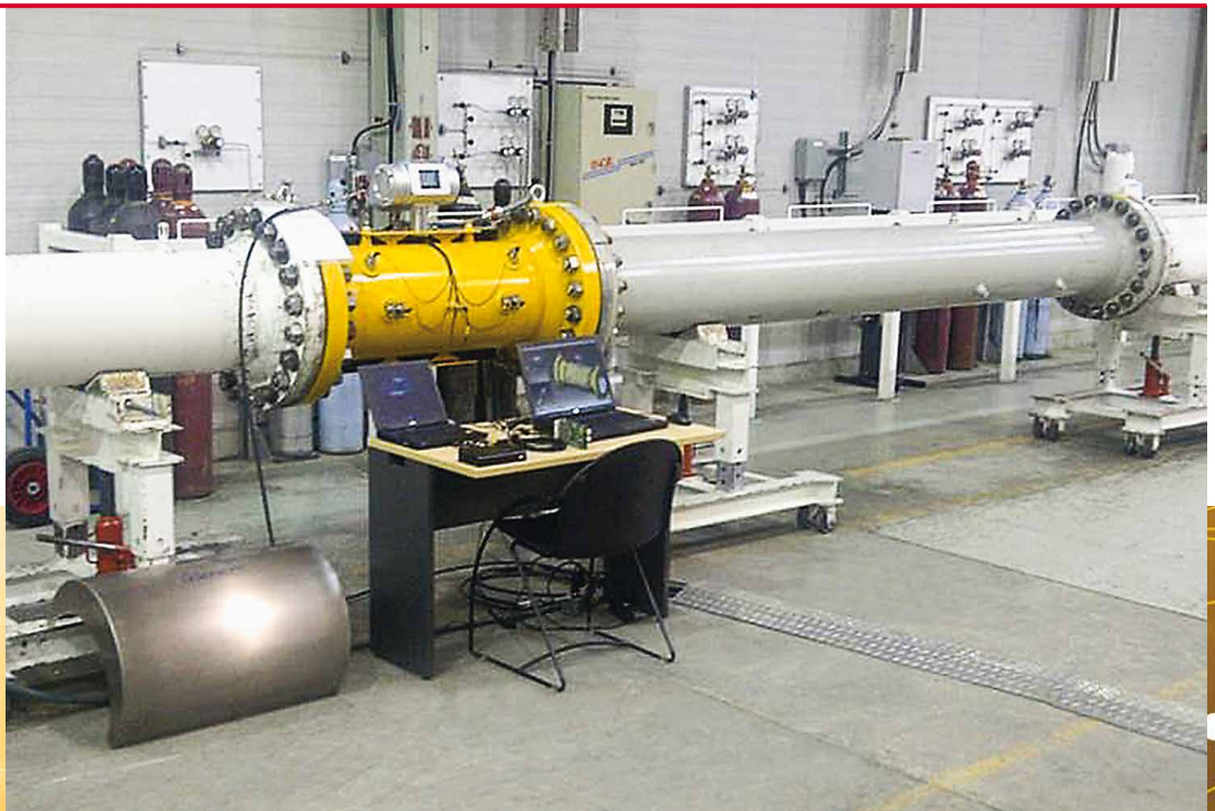
Transducer Replacement Testing
