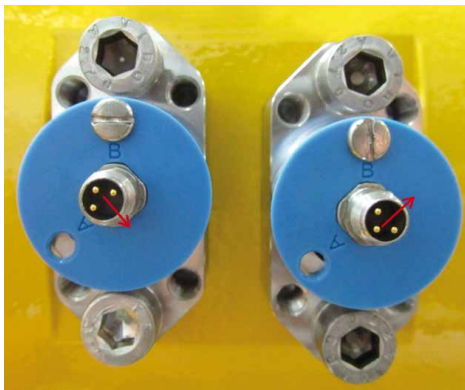
Fig. 1: Transducer Holder With Alignment Disc
