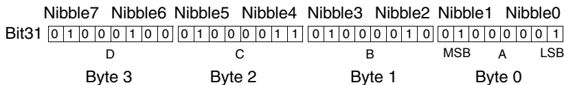
Figure 216. The ASCII codes for “ABCD” stored in an integer (packing = 4 characters per integer)
