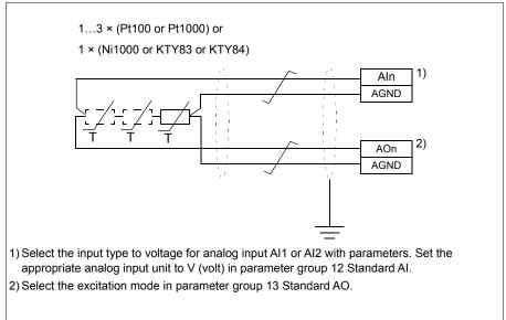
**WARNING!** As the inputs shown above are not insulated according to IEC 60664, the connection of the motor temperature sensor requires double or reinforced insulation between motor live parts and the sensor. If the assembly does not fulfill the requirement, the control unit I/O terminals must be protected against contact and must not be connected to other equipment or the temperature sensor must be isolated from the I/O terminals.
