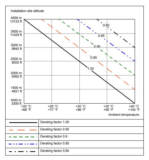
The altitude derating can be reduced if the temperature is below +40 °C, for example, if the temperature is 30 °C, the derating factor is 1 -  $1.5\% \cdot 10 = 0.85$ . You can reduce the output current by 35% instead of 40% at 4000 meter above the see level.
