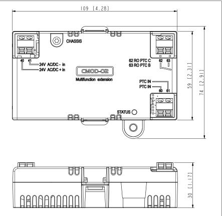
Installation: Into an option slot on the drive control unit
