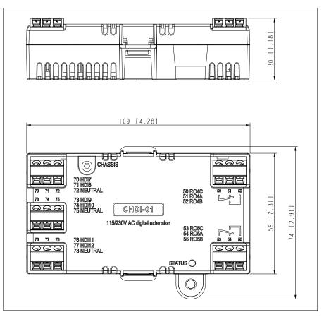
Installation: Into an option slot on the drive control unit
