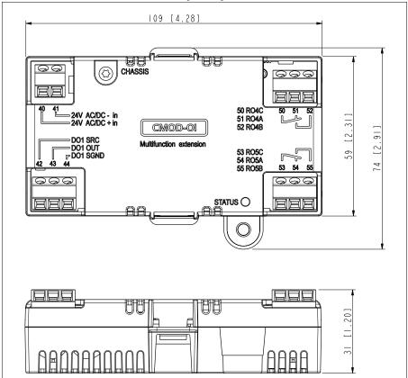
Installation: Into an option slot on the drive control unit
