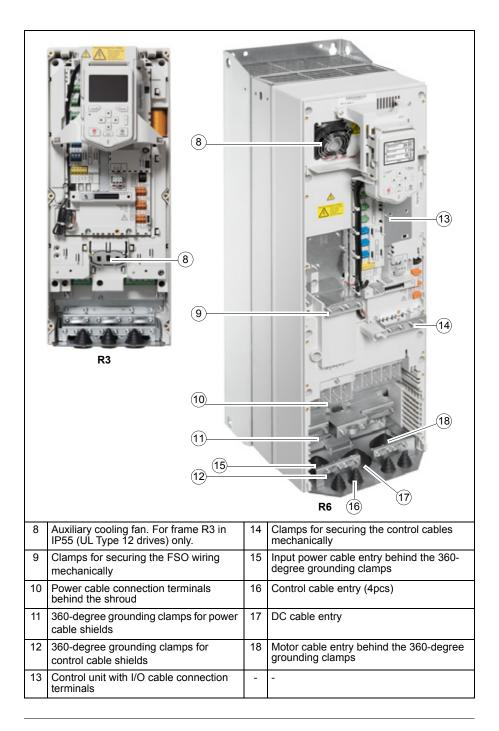
The main cooling fan is at the top of the drive in frame R3 and at the bottom in frames R6 and R8.
