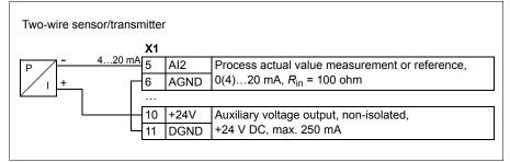
**Note:** The sensor is supplied through its current output and the drive feeds the supply voltage (+24 V DC). Thus the output signal must be 4...20 mA, not 0...20 mA.
