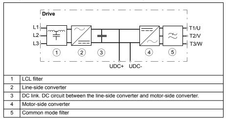
The figure below shows the simplified main circuit diagram of the drive.
