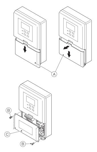
Figure 1 Removing lower cover
