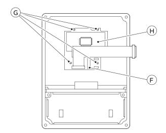
Figure 2 Removing transmitter front cover
