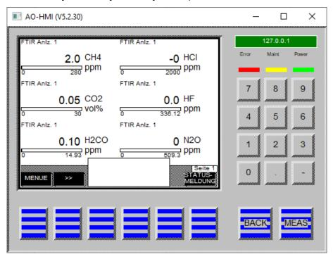
Figure 32 AO2000 Remote HMI
