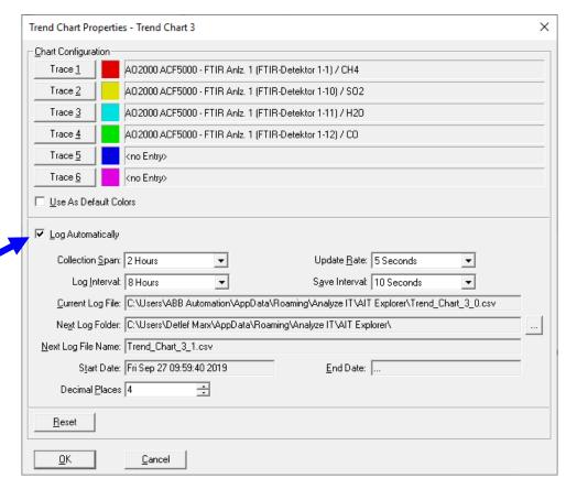
Figure 45 Enabling Automatic logging
