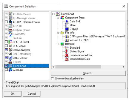
Figure 42 Enabling the Trend Chart Component
