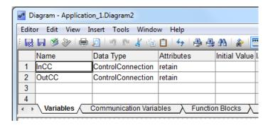
Figure 43. Variables for connecting the CCTemplate object in the diagram
