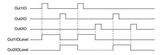
Figure 158. OutputIOLevel state diagram
