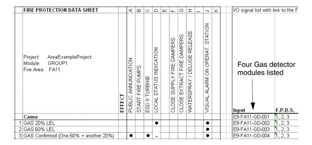
Figure 225. Part of the data sheet presenting information for Gas detection
