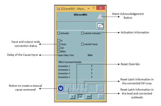
Figure 210. The Process Portal Faceplate of SDLevelM
