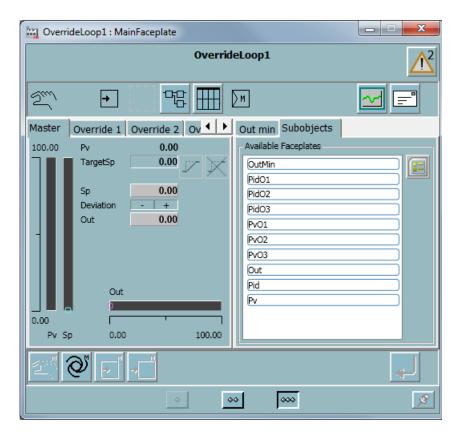
Figure 105. Extended faceplate of OverrideLoop displaying sub objects
