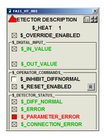
Figure 221. Parameter error indication in DetectorBool Interaction Window
