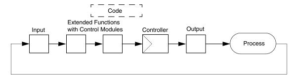
Figure 76. A control loop with all functions defined by control modules from the control libraries
