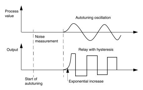
Figure 85. The process value oscillation
