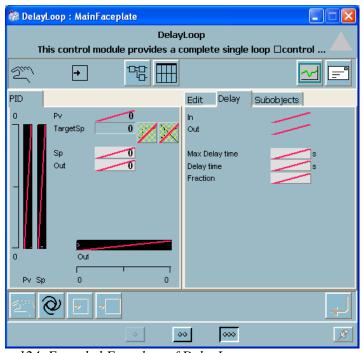
Figure 124. Extended Faceplate of DelayLoop
