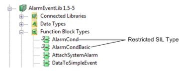
Figure 15. Restricted SIL marked objects in Project Explorer
