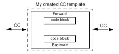
Figure 26. A control module prepared with two code blocks for handling forward and backward directions
