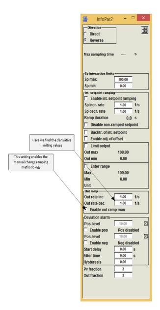
Figure 66. The interaction window of a PidCC or PidAdvancedCC
