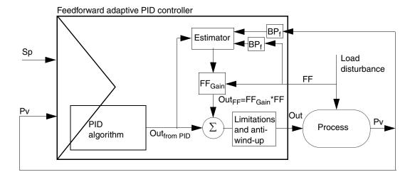
Figure 88. The principle of the feedforward adaptive PID controller
