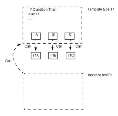
Figure 21. Execution of an instance of a template type with formal instances
