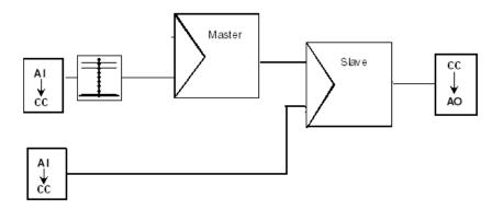
Figure 9. Cascade loop built from control modules
