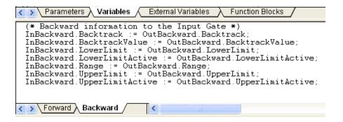
Figure 37. Programming code in the Backward code block
