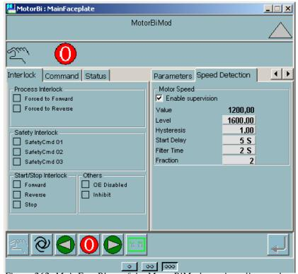
Figure 262. MainFacePlate of the MotorBiMod type in online mode
