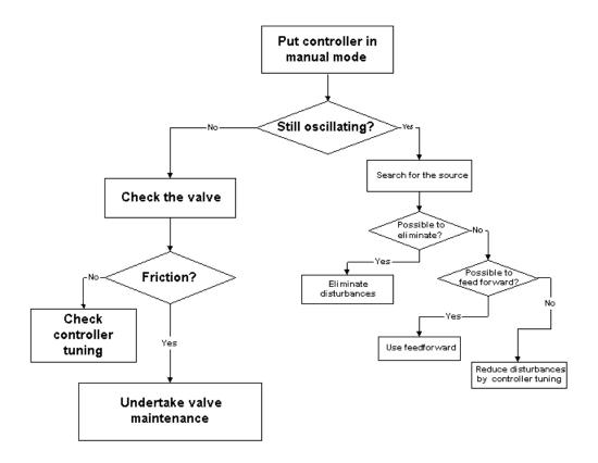
Figure 94. Flow chart for oscillation diagnosis
