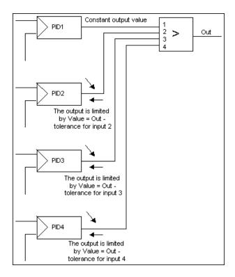
Figure 135. Example of a Max4CC control module with inputs from controller outputs
