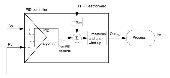
Figure 83. The feedforward principle in the controller
