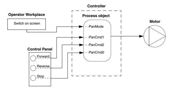
Figure 188. The Panel mode control diagram. A general solution for large applications, where the PanMode parameter is connected to an operator workplace
