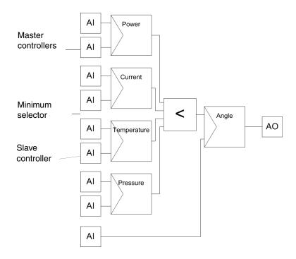
Figure 136. Example using control modules for override control in a heat pump using a minimum selector control module
