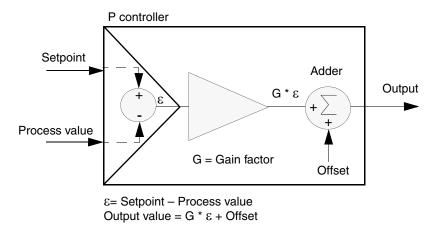
Figure 61. The basic P controller
