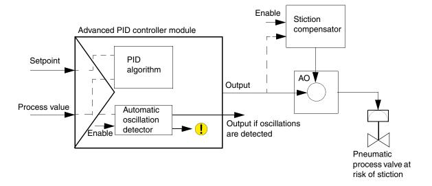
Figure 93. Principles for detecting and solving friction problems
