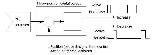
Figure 92. The principle of the three-position digital output function
