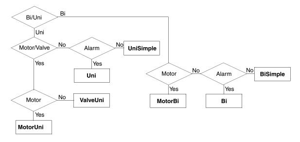
Figure 164. Flowchart of possible process object type choices
