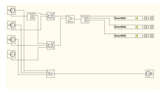
Figure 207. Configuration example of vote logic
