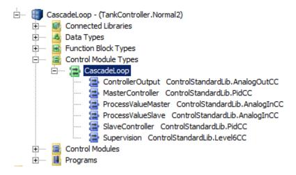
Figure 10. Cascade loop in Control Builder
