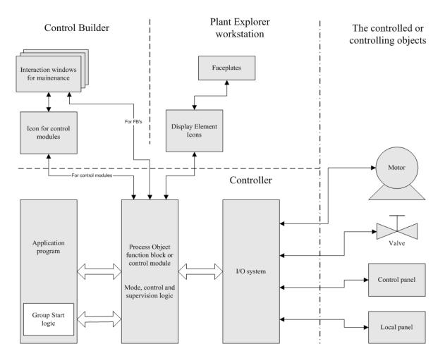
Figure 148. Relations between a function block or control module and the remote objects
