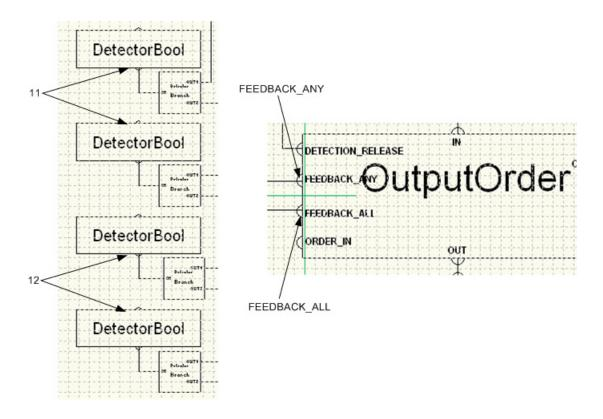
Figure 247. The location of Supply Fire Dampers Closed modules (11) and Extract Fire Dampers Closed modules (12)in the CMD Editor. The OutputOrder module with two feedback connections (depending on action)
