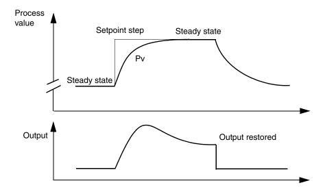
Figure 86. Setpoint step identification and output restoration
