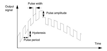
Figure 95. The stiction compensator signal is superimposed on the analog output signal
