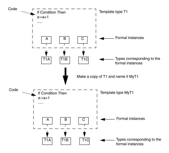
Figure 22. Copying a template type with formal instances
