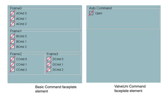
Figure 171. The basic Command faceplate element and the corresponding one in the ValveUni(M) type
