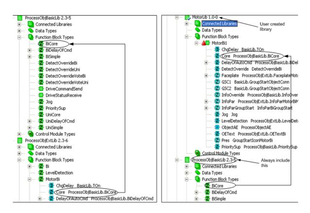
Figure 149. The core functionality in ProcessObjExtLib and in a user's self-defined library
