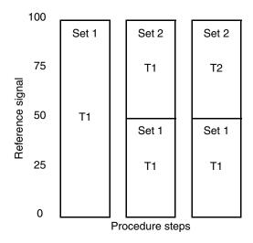
Figure 89. Example of the procedure for gain scheduling in two sets
