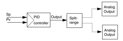
Figure 81. Example of split-range control where the output range from the controller is divided into two branches with different ranges
