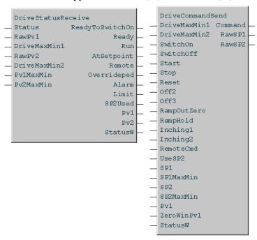
DriveStatusReceive are used to retrieve the status from a drive, after which the program or operator makes a decision based on this information. A command can then be issued to the drive using DriveCommandSend.
