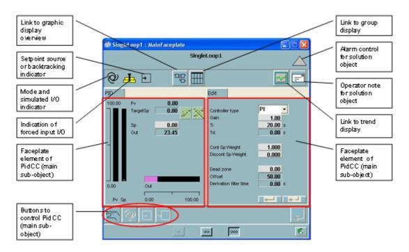
Figure 104. Extended faceplate of SingleLoop solution
