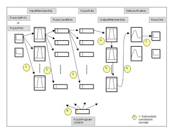
Figure 70. Sub-module connections in the fuzzy controller templates
