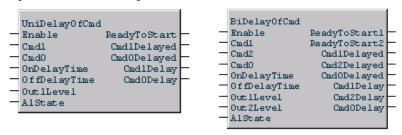
If, for example, a level detector informs an object to start, a disturbance pulse should not be able to start the object. The object shall not start until the detector delivers a reliable, constant signal stating that the start level is reached. If the object is a motor, this behavior is very important, in order not to wear it out.
