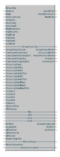
There is a parameter (*PanMode*), which is intended to be connected to an activation signal from the panel. If you connect PanMode to the panel it is still possible to use the button in the interaction window/faceplate to activate the Panel mode. It is, however, not possible to deactivate Panel mode from the interaction window/faceplate if it has been activated from the control panel.
