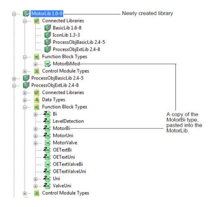
Figure 167. Copying of object types to a new library, MotorLib
