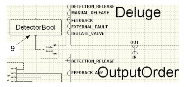
Figure 244. The location of Waterspray/Deluge Press Switch module in the CMD Editor
