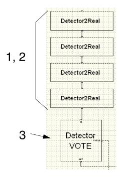
Figure 226. The four Gas detectors and a connected Vote module presented in the CMD Editor in FireAreaFA11
