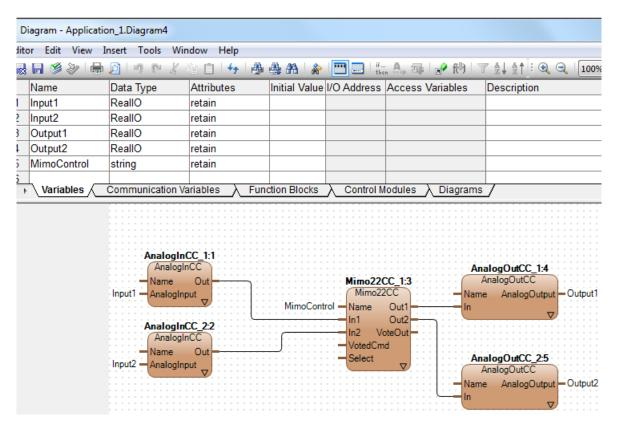
Figure 48. Mimo22CC connected in diagram editor
