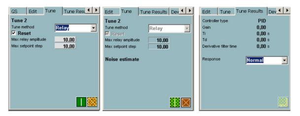
Figure 73. Autotuning in a PidAdvancedCC control module
