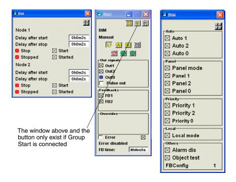
Figure 163. Control Builder interaction windows for Bi(M)
