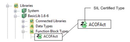
Figure 14. SIL marked object in Project Explorer
