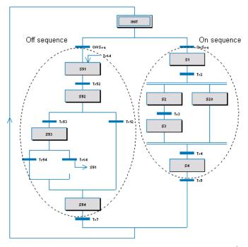
Figure 197. SFC structure configuration example
