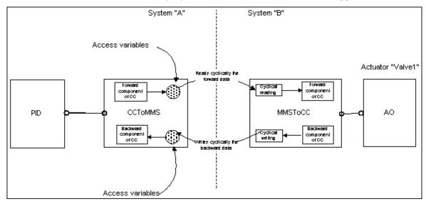
Figure 59. ControlConnection using control modules
