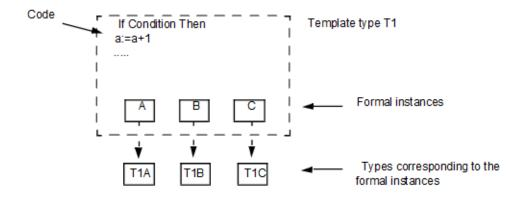
Figure 20. Template type with formal instances
