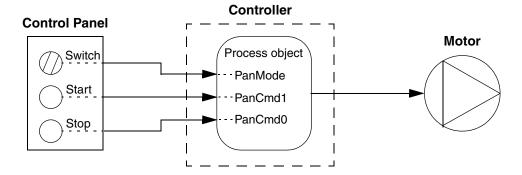
Figure 185. Control steps in Panel mode. This solution is recommended for small applications, where all three panel parameters are connected from a control panel
