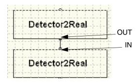
Figure 229. A graphical connection to the next Detector2Real module
