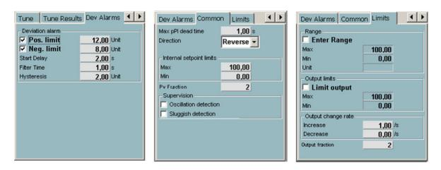
Figure 74. The settings of deviation alarms, common and limit settings in a PidAdvancedCC control module
