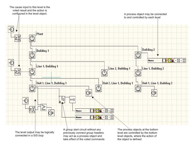
Figure 208. Level Usage Example
