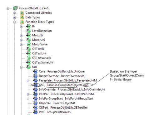
Figure 16. Uni function block type, with sub types and formal instances
