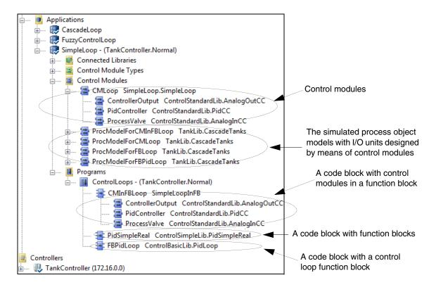
Figure 142. The four methods of designing an application and the simulated process
