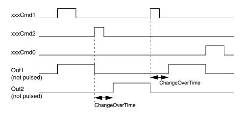
Figure 155. Change-over action state diagram
