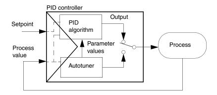
Figure 84. The principle of autotuning in a PID controller with the Autotuner function
