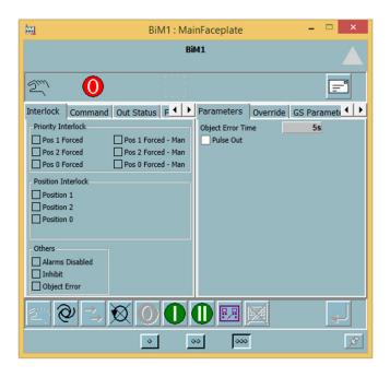
Figure 162. Example of extended faceplate (BiM)
