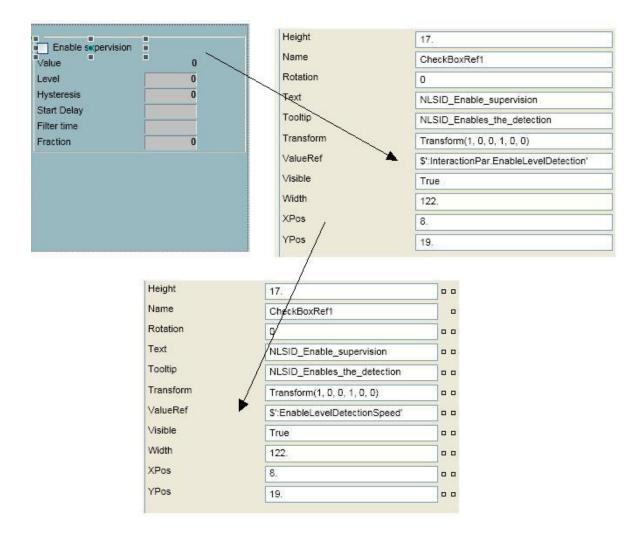
Figure 258. Changing the signals from EnableLevelDetection to EnableLevelDetectionSpeed
